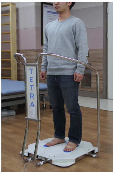
Fig. 1. Equipment for measuring parameters of postural control (The TETRAX biofeedback system).
