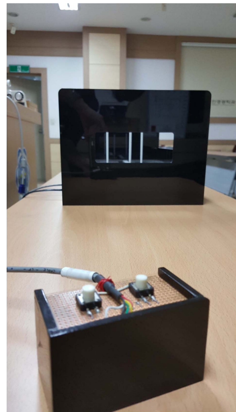
Fig. 1. Three-rods test system using automatic velocity system. Three-rods test system is automatically activated by the velocity control system. The instrument moves the middle bar of the three bars back and forth at a constant velocity 35 mm/sec, depending on the movement of the rail. The moving bar can be stopped by the controller with the stop button.
