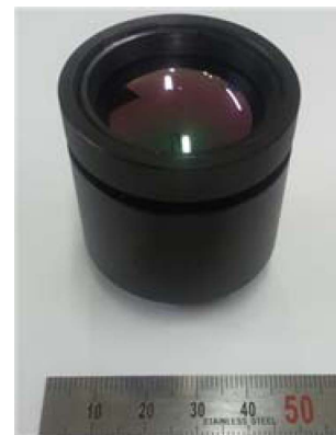
Fig. 8. External view of the assembled barrel with the optimized MWIR imaging optical system with 35 mm focal length.
