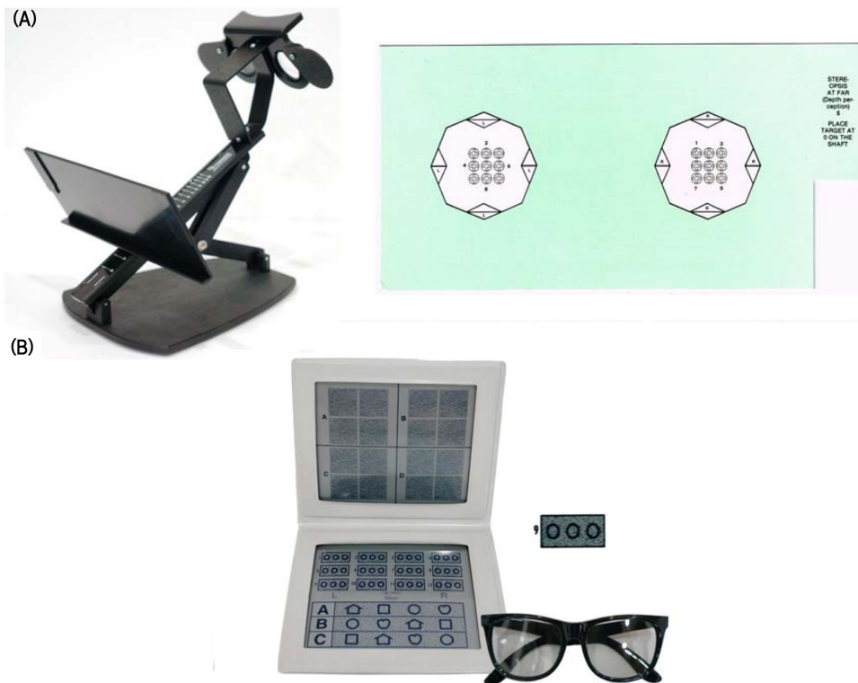
Fig. 2. Bernell-O-Scope (A) and Random dot stereo acuity test with lea symbols (B).
