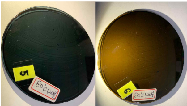
Fig. 4. Heat resistance of polarized lenses at 80°C.
