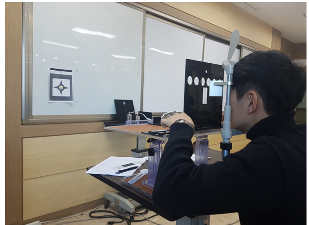
Fig. 2. Equipment used to measure the direction of the dominant eye and inset amount.
