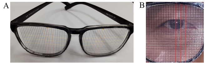
Fig. 1. Glasses attached a transparent grid film (A) and reflection point and lattices (B) for PD measurement.
