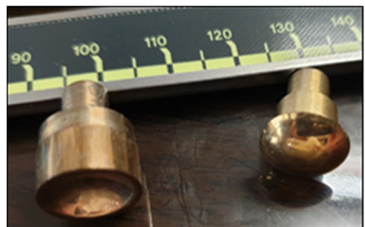
Fig. 5. Showing primary metal molds for contact lenses.
