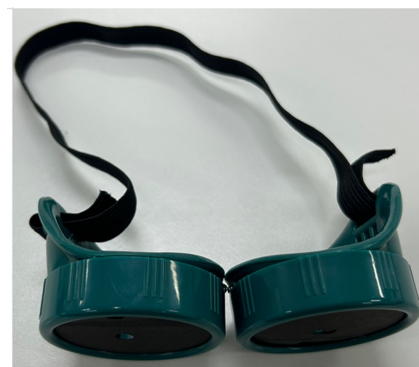
Fig. 2. The visual field restriction device was used to induce a 10-degree visual field.
