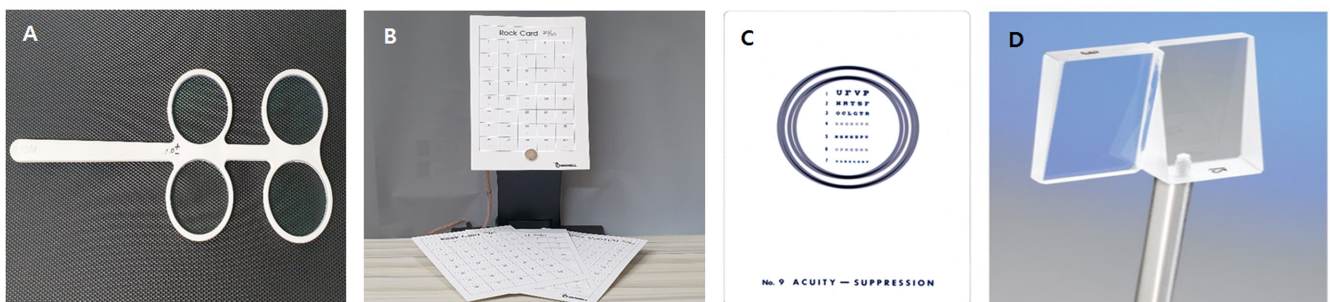
Fig. 2. Accommodative and vergence function measurement tools. A. Diopter flipper, B. Accommodative rock cards, C. Fixed vectogram, D. Vergence facility prism
