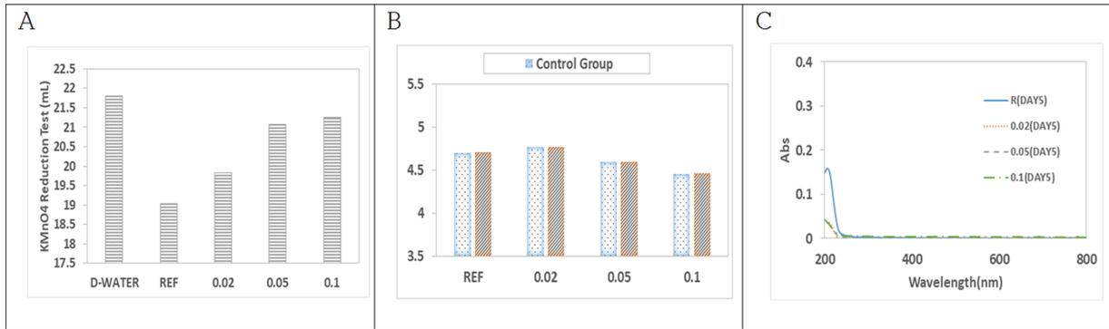
Fig. 8. Elution test of samples. A. KMnO<sub>4</sub> reduction test, B. pH test, C. Absorbance.
