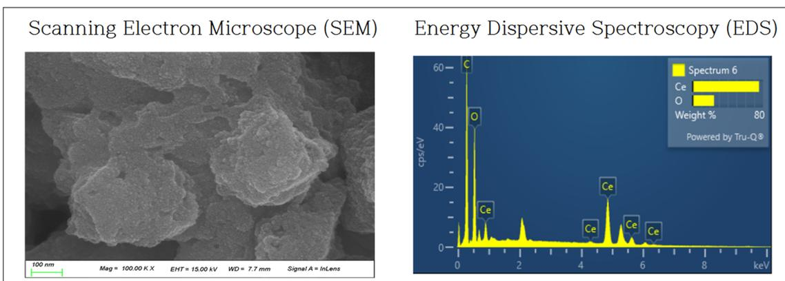
Fig. 2. Scanning electron microscopy and energy dispersive spectroscopy images of samples.
