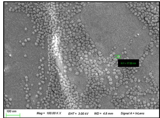
Fig. 3. Scanning electron micrograph of CeO<sub>2</sub> nanoparticles included in hydrogel lens.
