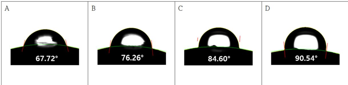
Fig. 6. Contact angle image of samples. A. Reference, B. 0.02% C. 0.05%, D. 0.10%.
