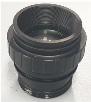
Fig. 8. External view of the assembled barrel with the optimized OLED imaging optical system having 23.0 mm focal length.
