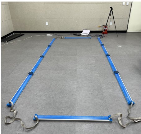
Fig. 1. Experimental setup of the OptoGait system used for gait analysis in this study.
