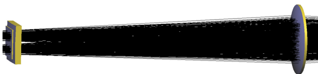
Fig. 7. Ray tracing through the final determined field lens set.
